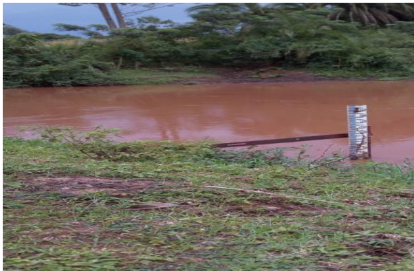
A working hydrological gauge on Kiminini tributary
